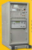
CE-TESTER 电磁兼容抗扰度测试仪 满足: IEC 61000-4-4 IEC 61000-4-5 IEC 61000-4-11
